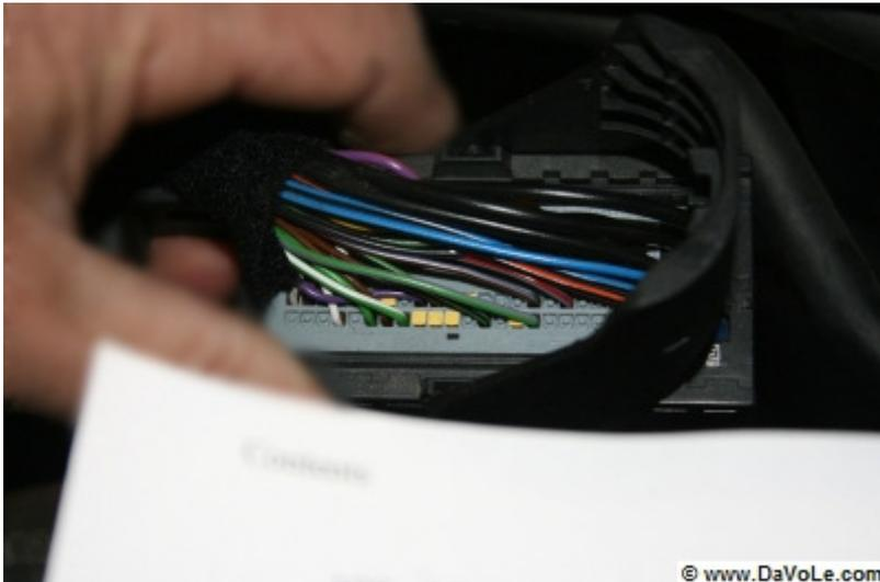
This is the upper side of the M010 connector (without protection).
