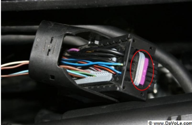
To unlock the connector, pull out the purple protection carefully.
