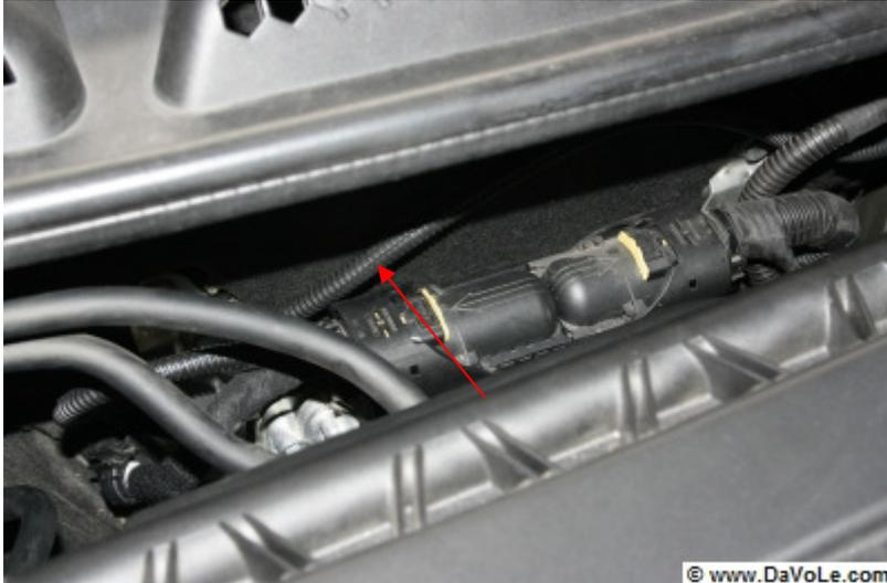
To protect the new cables I used some parts of the other cable harness, such as tubes and duct tape.
