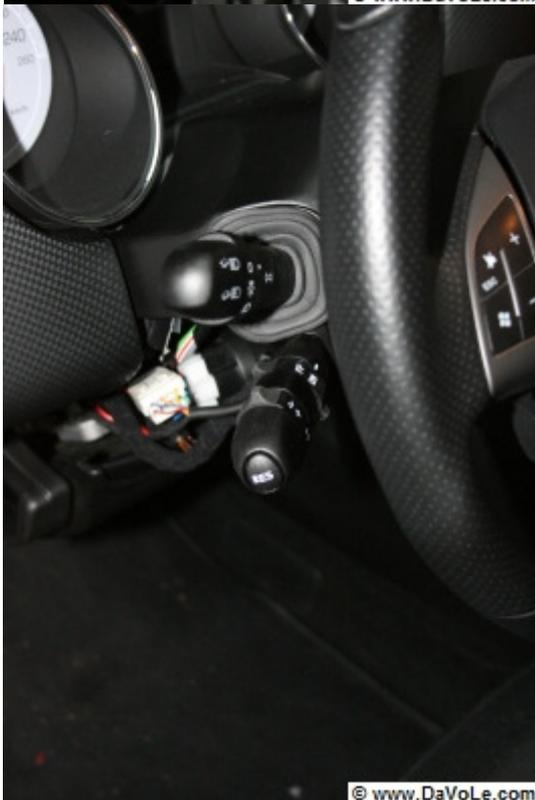
After laying the cables, I connected the power for the CC arm to the plus (+) of the ignition lock, using a 5A fuse.
