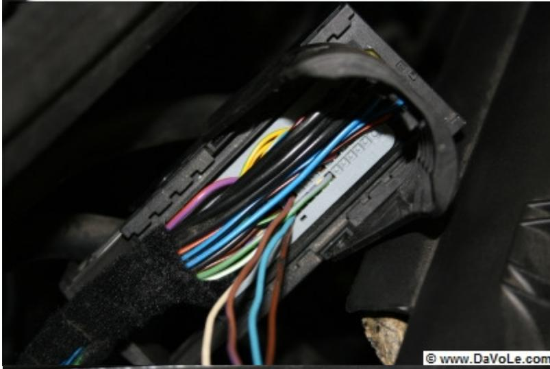
Remove the placeholders and unlock the connector (see next step) and stick in the (correct) cables, as you see in the scheme above.
