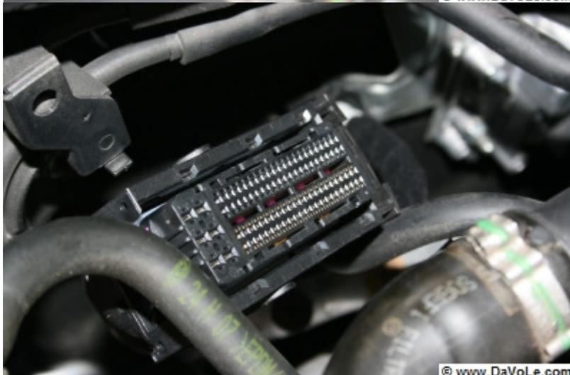
Turn the connector and check on the lower side if the slots (61,84,85,86) are occupied.
