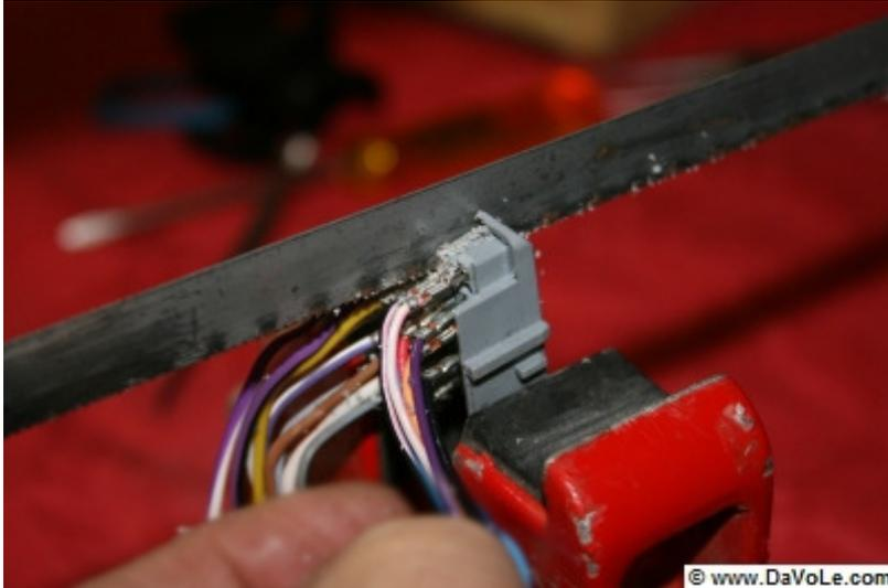
I took an old cable harness from another Fiat, and removed the cables including their sockets from a connector (similar to the M010 connector)
