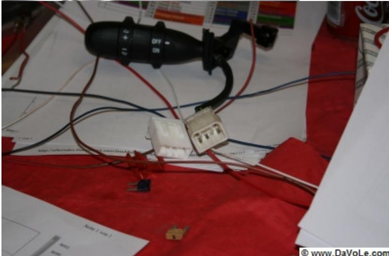
I needed to modify the CC arm, because I didn't have the corresponding connector.
