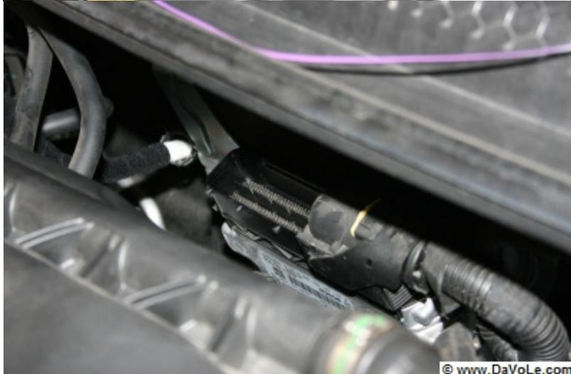
Remove the connector very carefully, to avoid deforming the pins or making contact between them.
