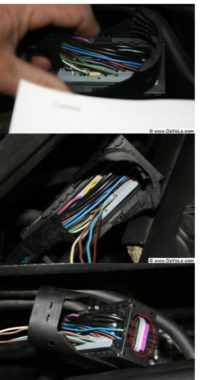
This is the upper side of the M010 connector (without protection).
