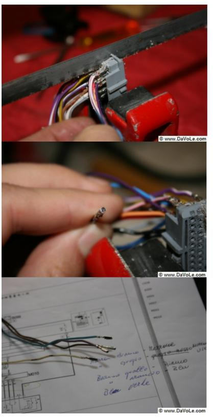
I took an old cable harness from another Fiat, and removed the cables including their sockets from a connector (similar to the M010 connector)
